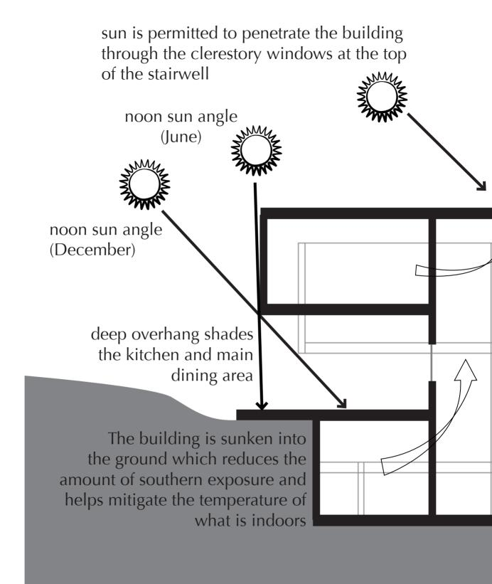
the stairwell acts as stack ventilation for the spaces, drawing heat and air out of the building
