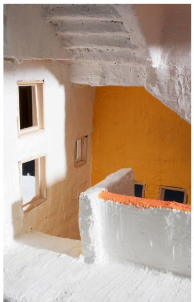
The stairs function on multiple levels in the design scheme. They act as a play space both in section and plan with small nooks and scaled levels. They also act as stack ventilation and a light well.
